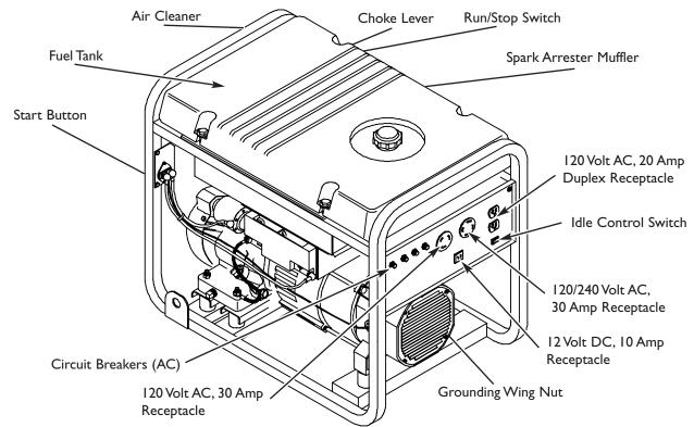
**12 Volt DC, 10 Amp Receptacle** — Recharge a discharged 12 Volt automotive type battery through this receptacle.
